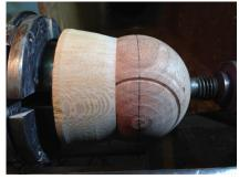
Put the sphere back in the four-jaw chuck, and using a beading and parting tool as a negative rake scraper, remove the wood down to the parting cut, the process is the same as used in making a regular sphere. In this case I like to bring the tail stock up to help hold the lid on (no point in the live center). Unlike when I make a sphere, I typically continue the rounding process past the center line. This leaves less to be removed using the jam chuck.
