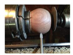
Now reverse the sphere into the jam chuck to finish rounding the sphere. Use the masking tape to hold the piece in the jam chuck just as with the sphere, only this time, make sure the tape covers the box joint. When finished rounding, do the final sanding.
