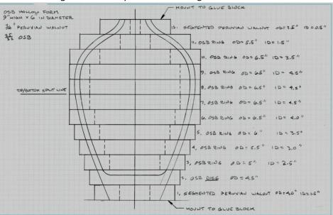
This is a construction and turning project, building the vessel up from both ends and joining them to do the final shaping. The drawing should be to scale, preferably 1:1 to allow setting calipers for measurement as you turn.
