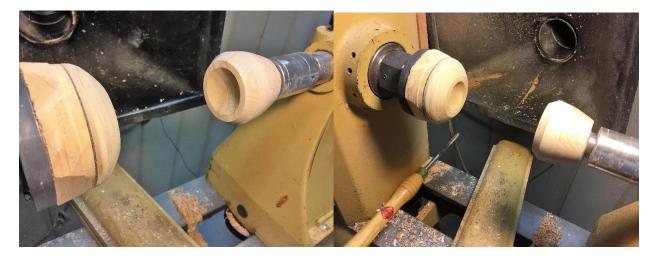
When using the cup chucks I often pad them with paper towels or leather to avoid marking the surface of the ball.
