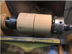
Step 3. I use a 1/16" parting tool to begin this process. On smaller diameter pieces, I compete the separation with the Parting tool. On larger pieces, I start with a parting tool and finish with a saw for safety.
