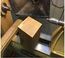
Blank size is optional...I have turned and hollowed balls as small as 2" and as large as 9". The maximum diameter is determined by your ball jig. The length of the blank must be longer than the diameter of the ball with enough length to accommodate a scroll chuck tenon at each end.
