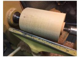
Step 2. Mount the blank between two scroll chucks and select the point at which the cylinder will be parted. This point should be near the center of the blank.
