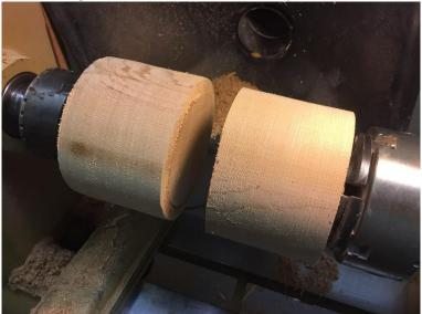
Step 5. The next step is to prepare a template to hollow a hemisphere in to each of the pieces. I use plastic lids saved from empty containers such as coffee cans, cottage cheese, etc. For larger diameters card stock, discarded file folders, etc. also work. Material must be ridged enough to be inserted into the hollow which will become the inside of the sphere.
