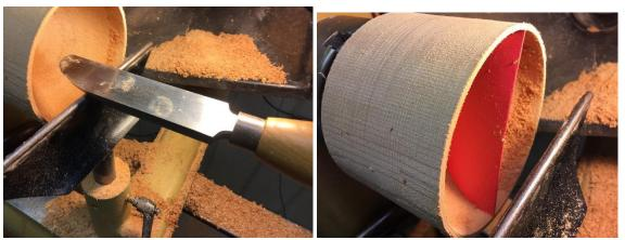
Step 9. Repeat this process for the other half and when satisfied with the hollowing and the rim surface glue 'm up! I use my lathe as a clamp and usually wait overnight before turning the outside of the sphere. I line up the grain and use a hose clamp to help line up the pieces. It can be removed from the lathe in 20 minutes or so you can get back to turning for empty bowls!
