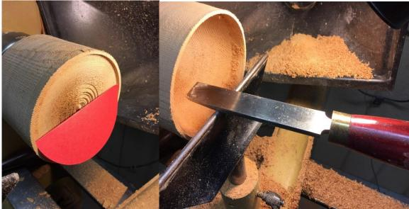
Step 8. Finish hollowing the hemisphere using the template to guide for accuracy. I use a bowl gouge and/or a round nosed scraper.
