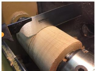
Step 4. After parting, true up the end of each half. This is an important step....the objective is to be able to match the two pieces back together with a seam that is nearly invisible.
