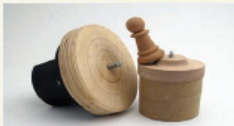
*Smaller-size shopmade screw chucks provide fast and easy mounting of small projects such as chessmen (right). Use a lag bolt if more support is needed, as shown in the example on the left that uses a faceplate and a scrap of plywood.*
