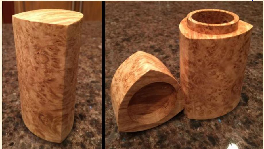
The demonstration will show how to setup a three sided off-center turning and cover the steps in making a friction fit lidded box. The techniques used in creating a three sided turning can be utilized in making a variety of projects and tends to be a good skill builder project for turners of all levels
