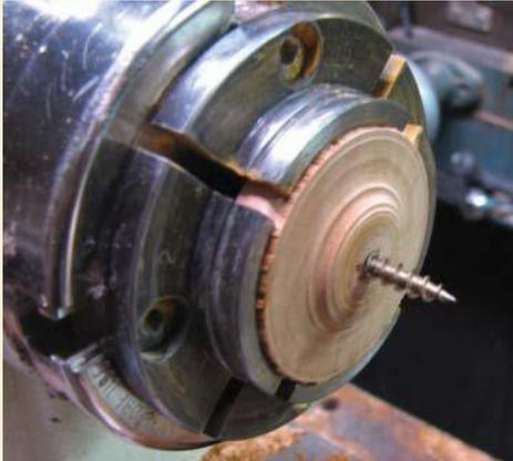
Once the epoxy has cured, the small size screw chuck is ready to use. Remount it into your chuck. Screw on your wood blank and turn to a shape of your choosing using gouge, skew and or scrapers.
