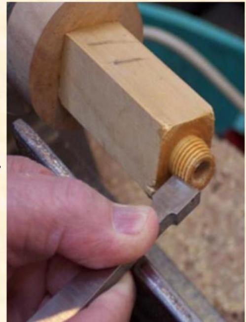
On this project, I drilled the 5/16" hole for the needles after I had chased the threads, but it can be drilled just as well before cutting the threads.
