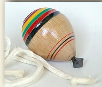
We are going to concentrate on the basic spinning top. Making a spinning top on a lathe is nothing more than spindle turning with the grain of the wood running parallel to the lathe bed. There is no one design; tops come in all shapes, sizes and material. Our goal will be to make a top that will spin for at least 60 seconds.
