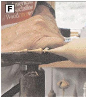
Next, use the roughing out gouge to start turning the icicle. You won't have the support of the tailstock to rely on, so take light cuts. I turn the smallest segment first (the tip of the icicle). I reduce the diameter with the roughing out gouge, and then refine the shape with a small skew and small spindle gouge as shown in Photo F.
