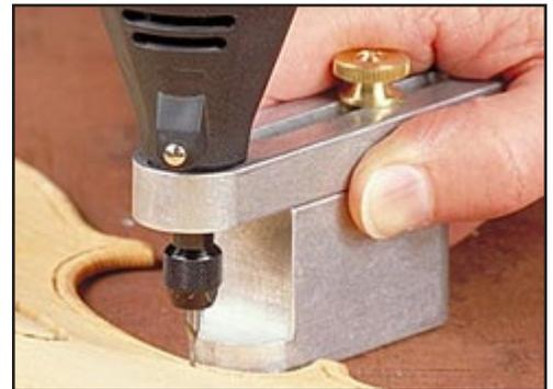
Dremel makes a little plastic router head that works well. Craftsman (Sears) makes a similar one shown here. I modify the basic design so the openings are large and drill a hole, glue in a fitting, and pump air at the cutting tip with an aquarium pump to clear away dust. Both Dremel and Craftsman can be found at many woodworking stores, Sears, and online from Widget Supply at [www.widgetsupply.com](http://www.widgetsupply.com).
