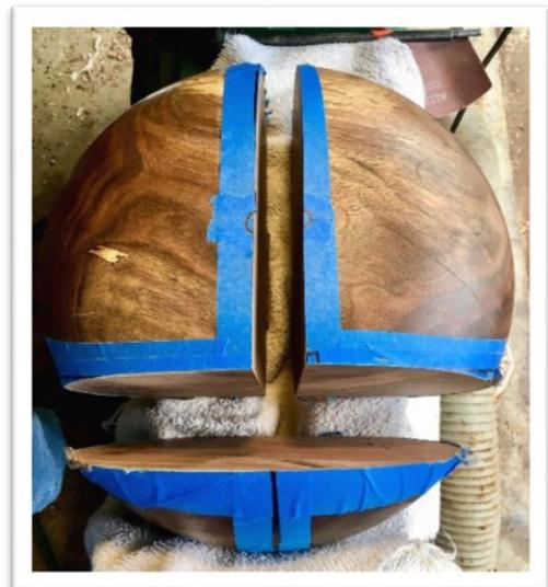
13. Remove painter's tape and finish the new unfinished wood surfaces by sanding, clear stain and then several coats of polyurethane. I found the use of painter's triangles extremely helpful when finishing with the polyurethane coats.
