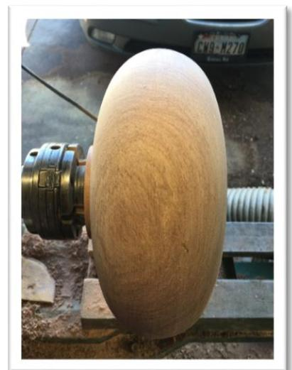
6. Once finished turning and while still on the lathe, sand as needed and desired.
