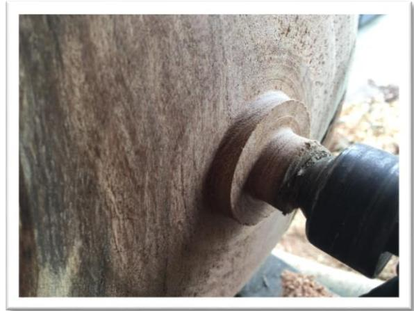
5. Remove from lathe, remove face plate, reverse piece and mount it back onto lathe with tenon in chuck.
