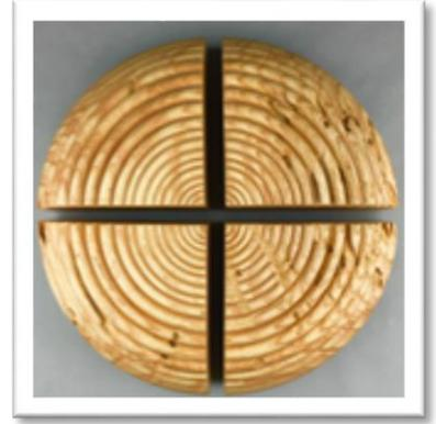
9. Once finish has cured, remove piece out of chuck and then remove tenon. I chose to remove the tenon with a sharp chisel. After tenon is removed, sand and then finish center section with clear natural stain and several coats of polyurethane.
