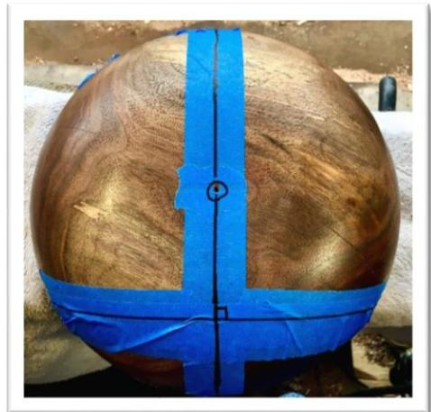
**11.** Put painter's tape on all of the underside surface and perimeter edges to protect the finish during the cutting process.
