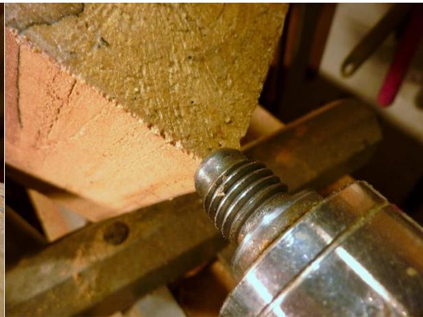
Figure 2: Cube secured in Hollow One-Way live center
