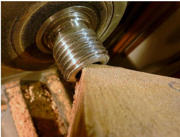
Figure 1: Corner inserted in Hollow Spindle
